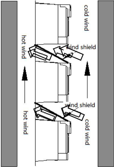
Note: when installing vertically, the wind shield must be added, otherwise it will cause mutual influence
