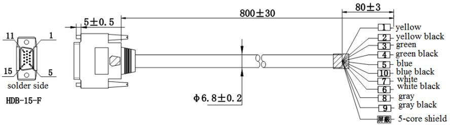
The user needs to define and connect the encoder signal pins according to the following core color and pin number:
