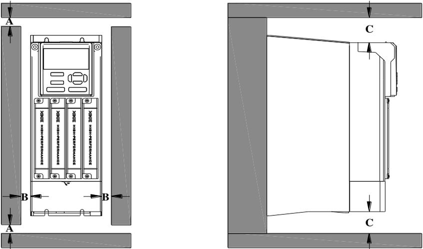
Note: the distance of A and B is more than 50 mm, and the distance of C is more than 100 mm.
