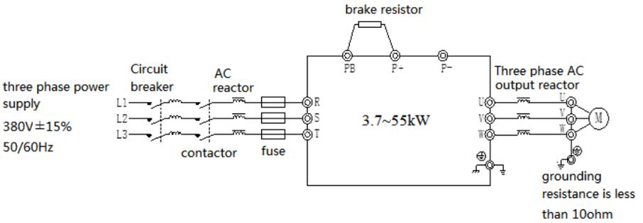
Note: circuit breaker, contactor, AC reactor, fuse, brake resistor and output reactor are optional parts. Please refer to chapter 6 for details.
