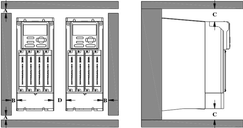
Note: the distance of A and B is more than 50mm, and the distance of C and D is more than 100mm.
