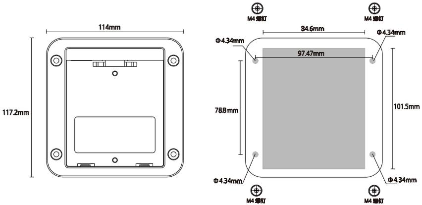
The gray area is the hollowed out part, and the middle hollowed out area is 84.6×101.5mm. The diameter of the four corner hollowed out area is 4.34 circle, and M4 screws and nuts are put in to fix the bracket on the panel.
