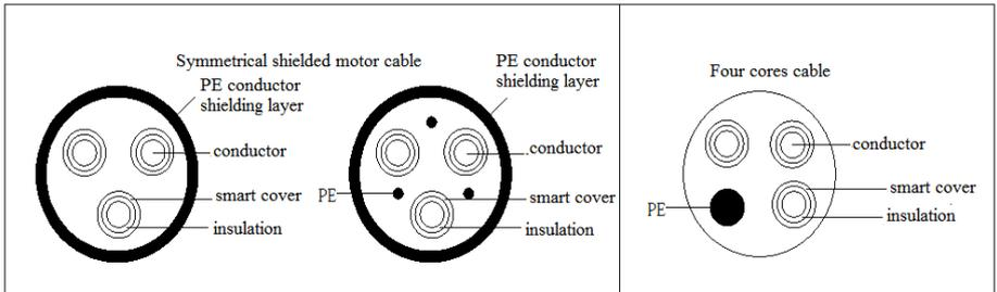
Note: if the conductivity of the shielding layer of the motor cable cannot meet the requirements, a separate PE conductor must be used.
