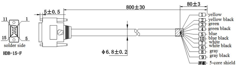
The user needs to define the signal pin connection of encoder according to the following core color and pin number:
