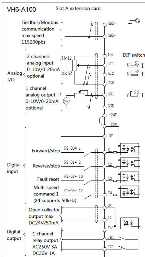
Note: VH6 series frequency converter has four card slots ABCD. Slot A I/O expansion card is standard installed when out of factory, slot BCD expansion card need to be selected by customers.
